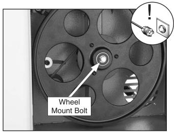
Figure 58. Example of wheel mount bolt.
